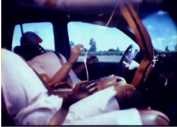
Figure 10. Max Seat rotation of a 2002 Chevrolet Trailblazer (11 degrees).
